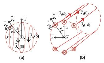
**Figure 1.** Current density distribution: (a) axisymmetric geometry in spherical coordinates, (b) plane geometry (infinite in z direction) in cylindrical coordinates. We adopt a unique angle notation for the two problems by substituting the usual  $\varphi$  (in the cylindrical coordinates) by  $\theta$ .
