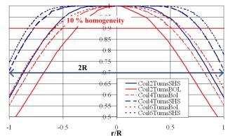
**Figure 8.** Magnetic field homogeneity profile on the *x* axis, comparison between Everett–Bolinger coil and SHS coil for two, four and six turns.
