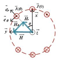
**Figure 2.** Representation of the magnetic field components  $\mathbf{H}$ ,  $\mathbf{H}_r$  and  $\mathbf{H}_{\theta}$  in the cartesian and cylindrical coordinates. Spherical coordinate representation is equivalent to the cylindrical one in a revolution near.
