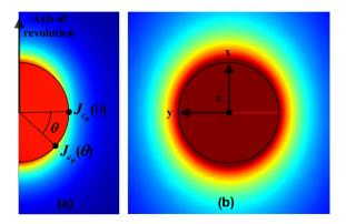
**Figure 3.** Magnetic field magnitude distribution of the ideal homogeneous coil (assuming  $cos(\theta)$  distribution of the current density along the circumference) performed on a numerical finite-element software: (a) case of a solid of revolution and (b) case of a 2-D plane infinite (along z) geometry. The colour scale is related to the magnitude of the magnetic field. The homogeneity of the colour is related to the homogeneity of the magnetic field.
